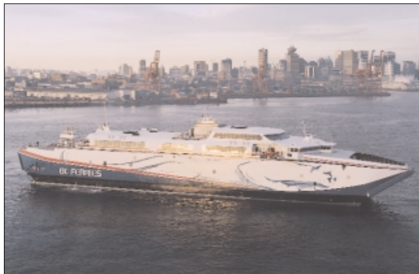
The extended bow of the fast ferry allows it to use existing BC Ferries docks
