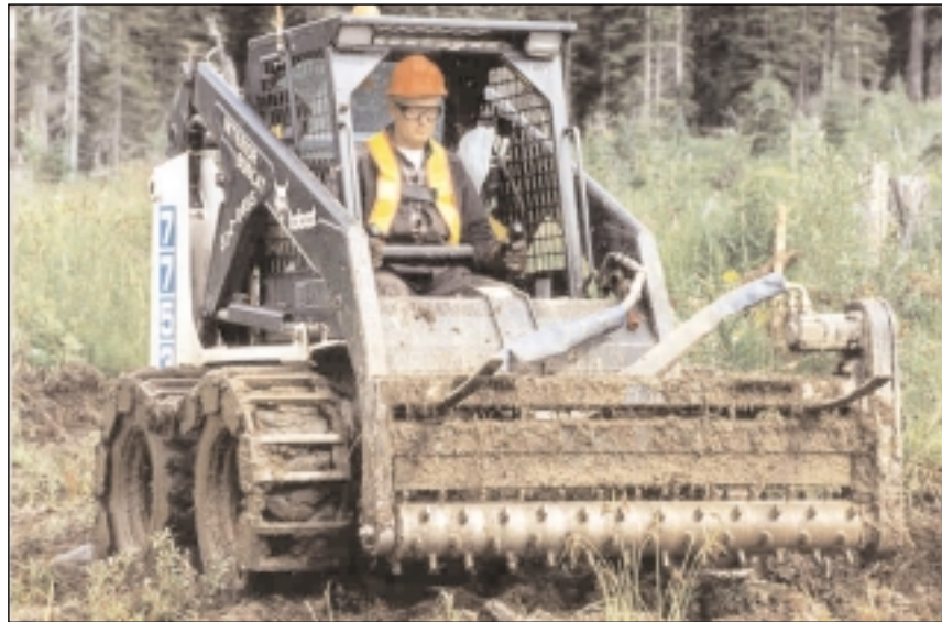
Bobcat operator churns soil that was once a landing for sorting and piling logs so that it can be replanted to productivity
