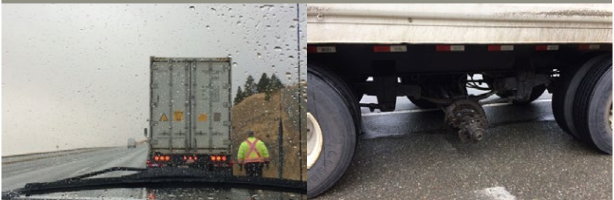
Exhibit 9: Truck missing wheel while driving on provincial highway
